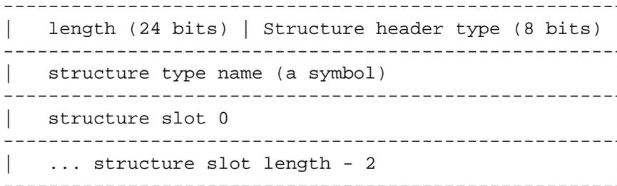
The header word contains the structure length, which is the number of words (other than the header word.) The length is always at least one, since the first word of the structure data is the structure type name.
