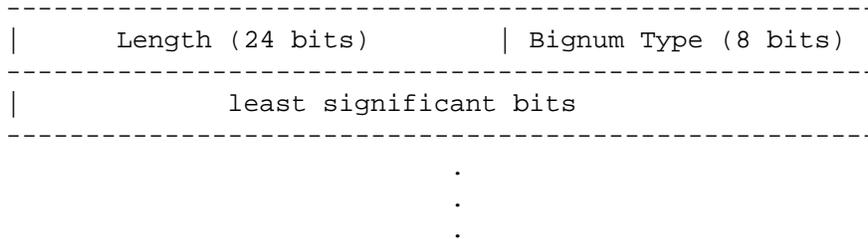
The elements contain the two's complement representation of the integer with the least significant bits in the first element or closer to the header. The sign information is in the high end of the last element.
